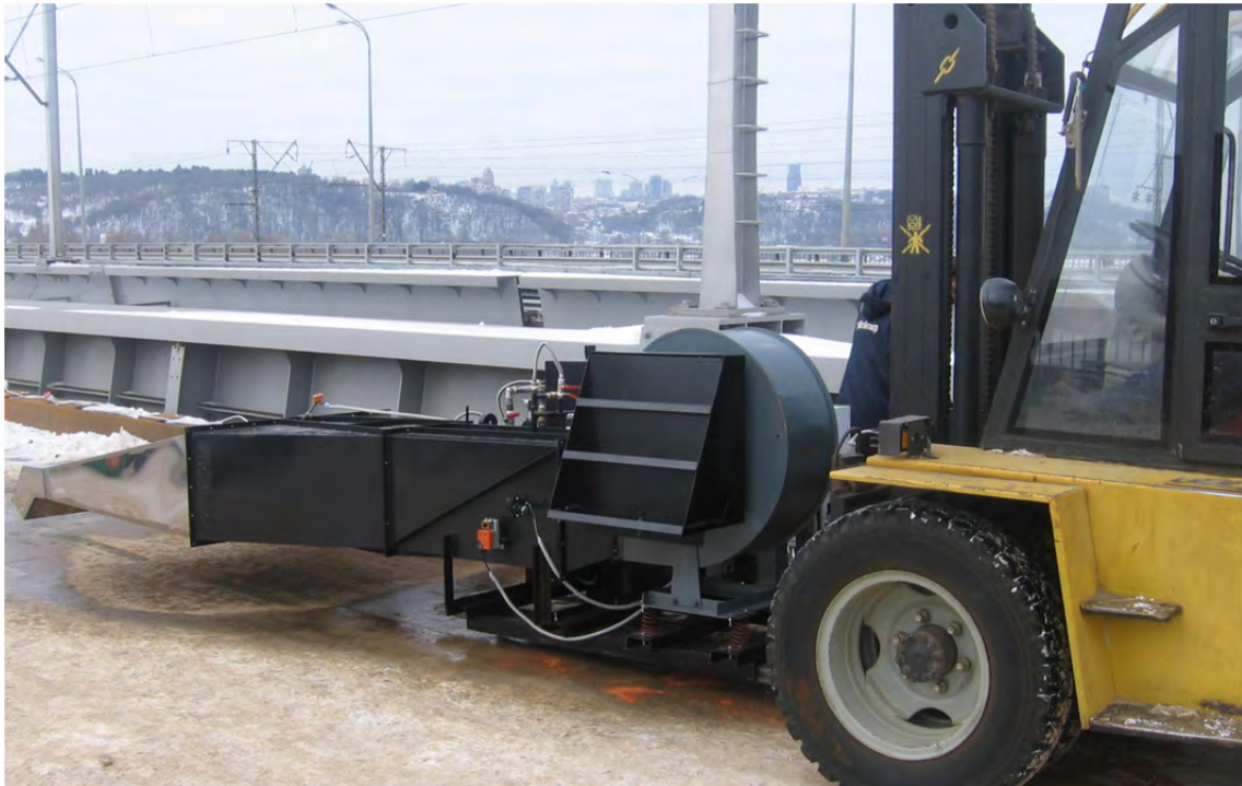
Mobile Heat Generator (2.2 MW) with a Diesel MD-Burner
